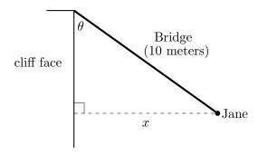
Note that the bridge is rigid and is 10 meters long. Assume that 2 seconds after the bridge snaps Jane is 8 meters from the cliff face (i.e. x = 8 in the figure above) and at that same moment the angle  $\theta$  between the bridge and the cliff is decreasing at a rate of 2 radians per second.
