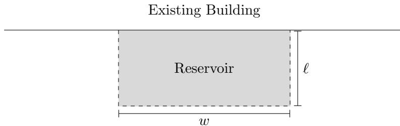
Three walls of the reservoir (dashed) and the floor of the reservoir (shaded) will be made of concrete. The cost for the concrete on the three walls is \$500 per meter of perimeter and the cost for the concrete for the floor is \$1000 per square meter.
