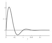
**b.** [7 points] If the mass is set in motion from equilibrium with an initial velocity v(0) = 8 m/s, the resulting motion is shown in the figure to the right, above. If we want the motion of the mass to not have any oscillatory characteristics, should we increase or decrease the value of c? If we do this, for what value of c will there first be no oscillation?
