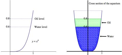
The aquarium contains water up to a level of y = 0.6 meters. There is a layer of oil of thickness 0.2 meters floating on top of the water. The water and olive oil have densities 1000 and 800 kg per m<sup>3</sup>, respectively. Use the value of g = 9.8 m per s<sup>2</sup> for the acceleration due to gravity.
